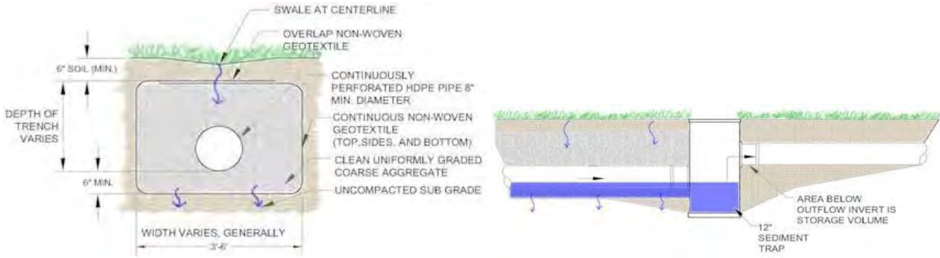
Figure 2: Infiltration Trench Diagram
