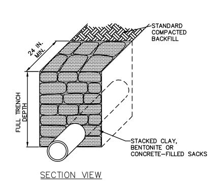
4. ACCUMULATED SEDIMENT SHALL BE REMOVED WHEN IT REACHES HALF THE ABOVE GROUND HEIGHT OF THE SOCK AND DISPOSED AS STATED IN THE RECYCLING AND
