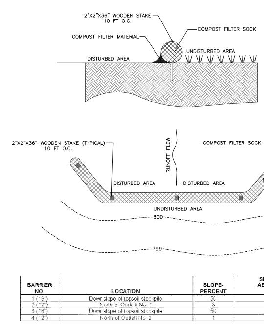
1. SOCK FABRIC SHALL MEET THE STANDARDS OF TABLE 4.1 (PAGE 63 OF THE PADEP EROSION AND SEDIMENT POLLUTION CONTROL MANUAL MARCH 2012). 2. COMPOST FILTER SOCK SHALL BE PLACED AT EXISTING LEVEL GRADE. BOTH ENDS OF THE SOCK SHALL BE EXTENDED AT LEAST 8 FEET UPSLOPE AT 45 DEGREES TO THE MAIN SOCK ALIGNMENT. STAKES MAY BE INSTALLED IMMEDIATELY DOWNSLOPE OF THE SOCK IF SO SPECIFIED BY THE MANUFACTURER.
